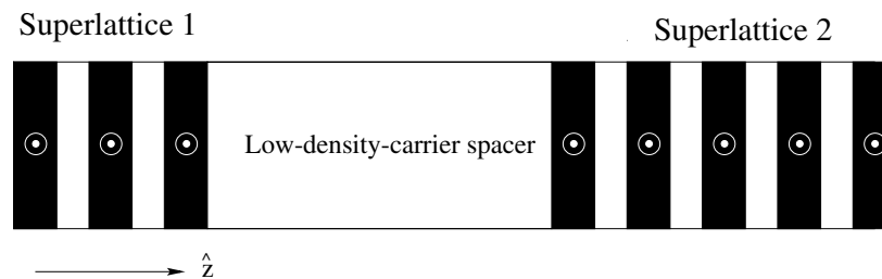
Figure 1. A schematic representation of the heterostructure showing the injector and collector magnetic superlattices, joined by a low-carrier-density spacer. The symbols \odot indicate the magnetization directions of the magnetic layers.
